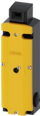
Safety position switch with tumbler Locking force 2600 N 5 directions of approaches Spring-locked Auxiliary release on front Magnet voltage 230 V AC Monitoring actuator 2 NC/1 NO Monitoring magnet 2 NC/1 NO Supplied without actuator. Actuator 3SE5000-0AV0. please order separately
