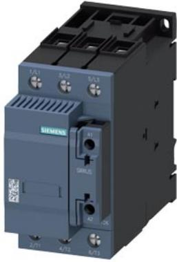
capacitor contactor, AC-6b 50 kVAr, / 400 V, 3-pole, 230 V AC, 50 Hz, auxiliary contacts: 1 NO + 1 NC, screw terminal, size: S2
