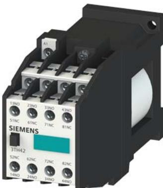
Contactor relay, 53E, DIN EN 50011, 5NO + 3NC, screw terminal DC operation 24 V DC
