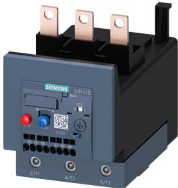
Overload relay 45...63 A Thermal For motor protection Size S3, Class 10 Contactor mounting Main circuit: Screw Auxiliary circuit: spring-type terminal Manual-Automatic-Reset
