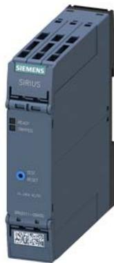
Thermistor motor protection relay Standard evaluation unit 22.5 mm enclosure Spring-type terminal 2 change-over contacts US = 24 V-240 V AC/DC Manul/Remote-Reset with ATEX approval 2 LEDs (READY/TRIPPED) galvanic isolation Test/reset button Wire break monitoring Short circuit monitoring
