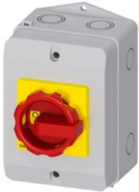
SENTRON, Switch disconnector 3LD, emergency switching-off switch, 3- pole, Iu: 25 A, operating power / at AC-23 A 400 V: 9.5 kW, Molded plastic encapsulation for metric cable gland, 1 NC, 1 NO, rotary operating mechanism, red/yellow
