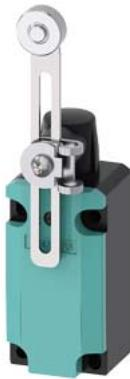
Position switch Metal enclosure 40 mm according to EN 50041 Device connection 1x (M20 x 1.5) 1 NO/1 NC quick action contacts Rotary actuator right/left adjustable with adjustable-length Metal lever 100 mm long and Stainless steel roller 19 mm
