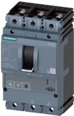
circuit breaker 3VA2 IEC frame 250 breaking capacity class M  $I_{cu}=55\text{kA}$  @ 415V 3-pole, motor protection ETU350M, LSI,  $I_{n}=160\text{A}$  overload protection  $I_r=63\text{A}\dots160\text{A}$  short-circuit protection  $I_{sd}=3\dots15 \times I_r$ ,  $I_i=15 \times I_n$  nut keeper kit
