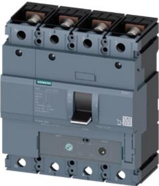
circuit breaker 3VA1 IEC frame 250 breaking capacity class S Icu=36kA @ 415V 4-pole, line protection TM240, ATAM, In=250A overload protection Ir=175A...250A short-circuit protection Ii=5...10 x In N conductor protection 100% nut keeper kit
