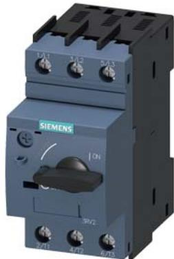
Circuit breaker size S00 for transformer protection A-release 0.9...1.25 A N-release 26 A screw terminal Standard switching capacity
