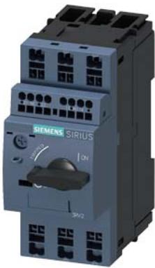
Circuit breaker size S00 for motor protection, CLASS 10 A-release 0.22...0.32 A N-release 4.2 A Spring-type terminal Standard switching capacity with transverse auxiliary switches 1 NO+1 NC
