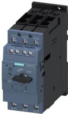
Circuit breaker size S2 for motor protection, CLASS 10 A-release 35...45 A N-release 650 A screw terminal Standard switching capacity with transverse auxiliary switches 1 NO+1 NC
