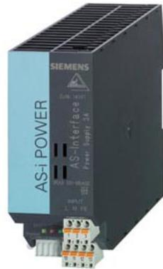
AS-i Power 3A 120 V/230 V AC AS-Interface power supply unit, IP20 IN: 120 V / 230 V AC OUT: AS-i, 3 A (30 V DC), IP20 with integrated ground fault detection, with integrated overload detection with AS-i data decoupling
